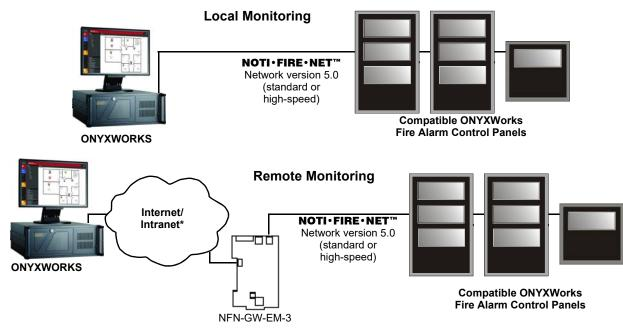
\* A UL listed Ethernet (TCP/IP) switch is required between a shared-IP network and the ONYXWorks equipment. Contemporary Control Systems, Inc. (www.ctrlink.com) has several UL864 recognized switching hubs.
