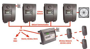
E³Point outputs directly to BACnet or other BAS. Alarms, strobes and horns are activated through BAS with link to DCV/HVAC controls. This system design supports new and retrofit installations for large buildings, and can couple with a controller to effectively integrate wired and wireless system components. A relay output is provided as an option for activating ventilation directly (e.g. when fan is located in close proximity to detector).
