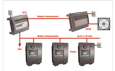
Supports Modbus protocol to daisy-chain  $E^3$ Point detectors, providing up to 96 points of monitoring on a serial bus. Excellent option for controller-based (VA301C) installations common in larger applications. A relay output is provided as an option for activating ventilation directly (e.g. when fan is located in close proximity to detector).
